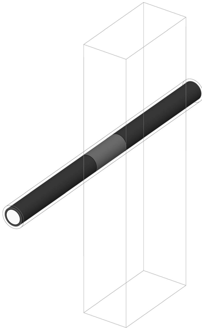
FIG. 2. An oblique view of the simulations of ^{153}\text{Sm} and ^{90}\text{Y} . The block of tissue is rendered as a wireframe of a rectangular prism that is 5 cm thick, 10 cm wide and 30 cm high. The segment of the bone simulating the lesion is the brighter area in the center of the cylinder that is in contact with the tissue block.
