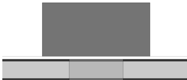
FIG. 1. A top-down view of a cross-section through a central plane of the simulation of the treatments with 153 Sm and 90 Y. The rectangle at the top of the figure is the block of tissue, which is pressed up against the treated limb. It is 5 cm thick, 10 cm wide (in the direction of the limb) and 30 cm high (perpendicular to the direction of the limb). The inner core of the simulated bone has a radius of 8 mm and the material properties of trabecular bone while the 2-mm-thick outer sheath has the material properties of cortical bone. A 2.5-mm-thick sheath with the properties of tissue surrounds the bone. For 153 Sm and 90 Y, the radionuclide was uniformly distributed within both the trabecular and cortical portions of the central segment of the bone in order to simulate a lesion. For 153 Sm the portions of the bone that are adjacent to the portion simulating the lesion had one-tenth of the activity of the central portion; whereas for 90 Y the bone outside of the lesion contained no radioactivity.
